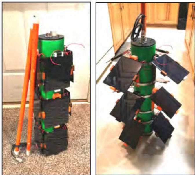
Digipeater closed for transport (left) and open for use (right).
