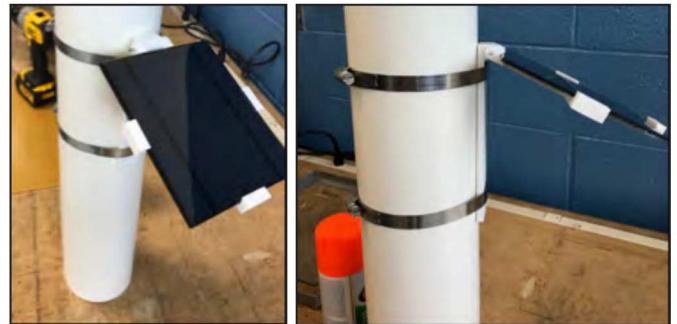
Mounting assembly for the solar panels.
